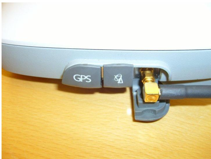
**Figure 5. Connecting to the Thuraya IP terminal via the active external antenna connector.**
