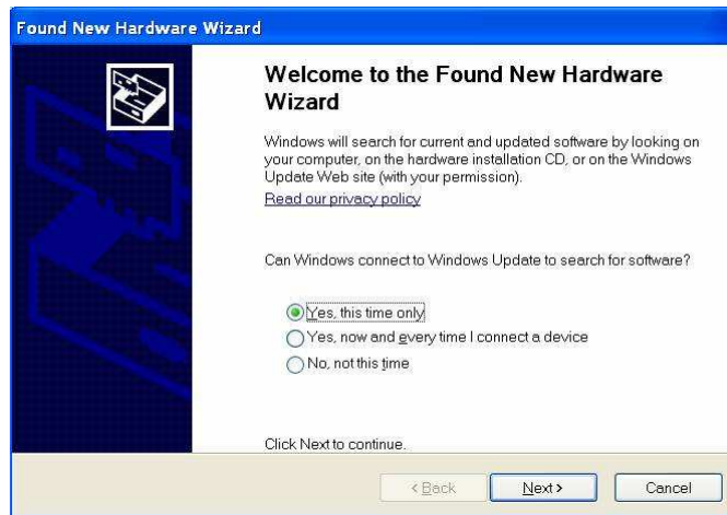
Figure 8. The "Found New Hardware Wizard". Enable the Windows Update search and press "Next".
